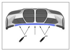
Position the Sterckenn splitter properly on the bumper using genuine OEM mounting screws.
