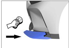
Position the side splitter properly on the edge of the bumper.
