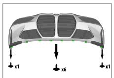
Remove 8 OEM mounting screws.
