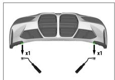
Remove 2 OEM plastic rivets from the side bumper trim.
