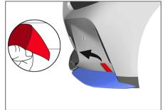
Remove the adhesive backing film just enough to form small tabs.
