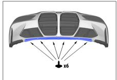
Install all 6 OEM screws that were removed before.
