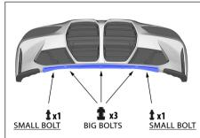
Install 5 bolts that are attached to this mounting kit.
