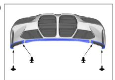
Install 2 OEM screws and 2 OEM plastic rivets that were removed before.
