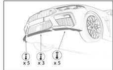
Install 13 screws that are attached to this mounting kit.
