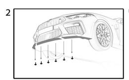
Remove OEM mounting screws.
