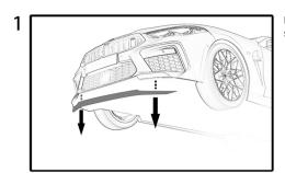
Remove OEM center cover and side splash shields.
