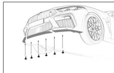
Install all 8mm screws that were removed before.
