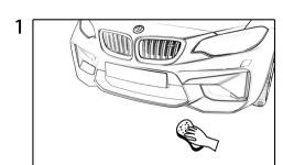
The areas being bonded must be completely dry, clean and free from wax or grease.
