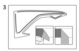
Remove the adhesive backing film just enough to form small tabs.
