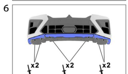
Install 6 plastic rivets that are attached to this mounting kit. (mounting diagram)
