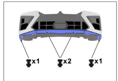
Install 4 M6 bolts that are attached to this mounting kit. (mounting diagram)
