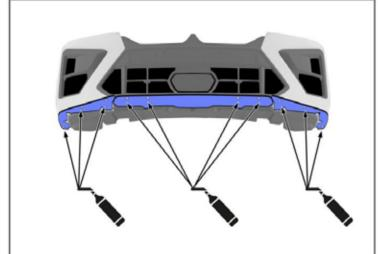
Mark all 10 not OEM spots necessary to drill the holes.
