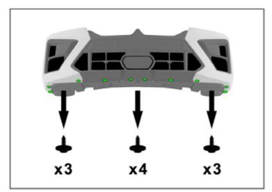
Front bumper doesn't need to be removed from the car to perform this installation.
