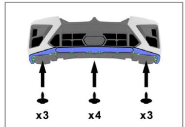
Position the Sterckenn splitter properly on the bumper using genuine 10 OEM mounting screws.
