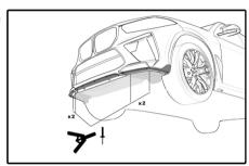
Install the 4 plastic rivets which are attached to this mounting kit.
