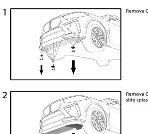
Remove OEM mounting screws.
