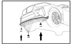
Install all the 8mm screws which were removed before.
