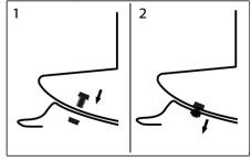
We suggest to slide the bolt from inside of the bumper first for easier positioning.
