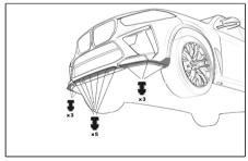
Install 11 screws which are attached to this mounting kit.
