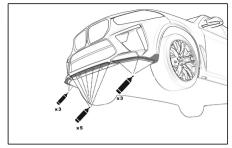
Position the Sterckenn splitter properly on the bumper using genuine OEM mounting screws.
