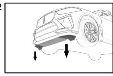
Remove OEM center cover and side splash shields.
