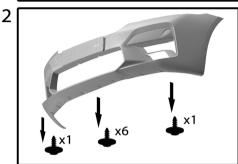
Remove OEM mounting screws
