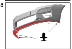
Install the 6 plastic rivets which were removed bofere this installation.
