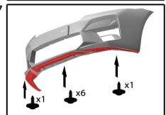
Install all the 8mm screws which were removed before.
