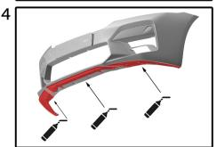
Position the Sterckenn splitter properly on the bumper using genuine OEM mounting screws.
