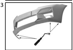
Remove 4 OEM plastic rivets for better access inside the bumper.
