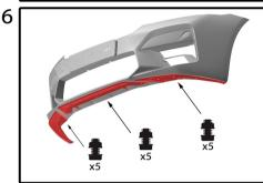
Install 15 screws which are attached to this mounting kit.
