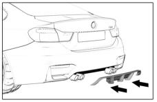
Align the Sterckenn diffuser tabs with the slots in the bumper. Then press the diffuser into the slots locking the diffuser tabs.
