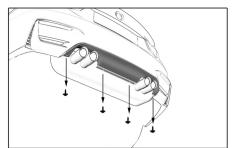
Remove the two 8mm screws on the outside corners of OEM diffuser and two 8mm screws holding the center of the exhaust heat shield. They are located near the muffler.
