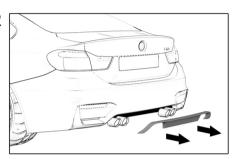
Carefuly pull back on the OEM diffuser, releasing the diffuser clips from the bumper. Remember to release the bottom diffuser clips located near the muffler.
