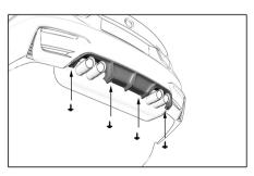
Align the Sterckenn diffuser mounting holes and install all four 8mm screws that were removed beofre. 5
